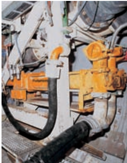
A KOV 1050 pumps the injection mortar behind the ring segment
