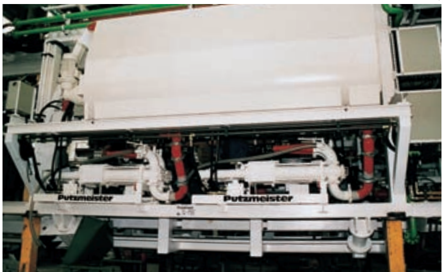
A KOV 1050 pumps the injection mortar behind the ring segment
