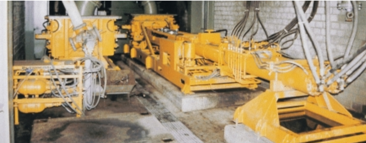
KOS 3080 backfilling pump at the Walsum mine
