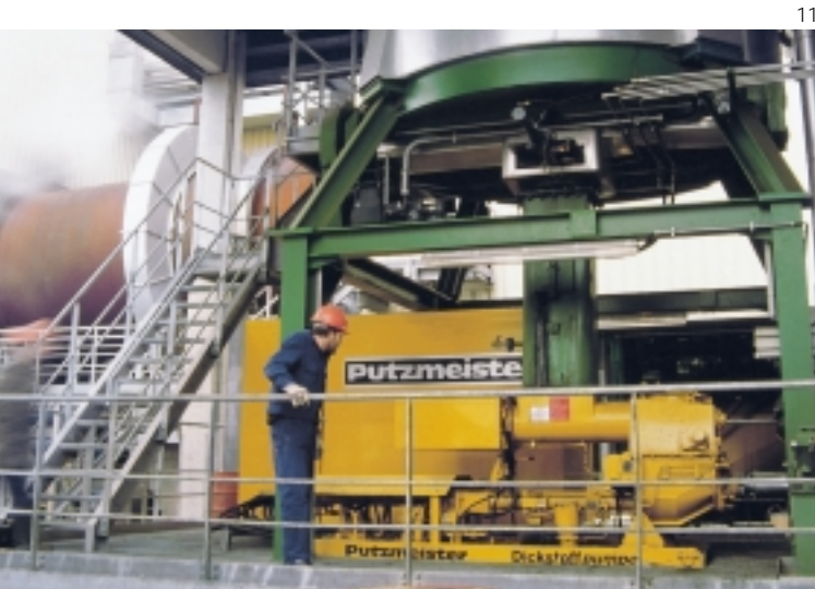
Paste-like hazardous waste being fed by the KOS 1030 into a rotary kiln at Schwabach hazardous waste treatment plant in Bavaria
