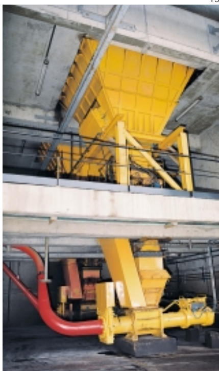
The EKO 14100 feeding the rotary kiln with shredded barrel waste at Tredi Salaise
