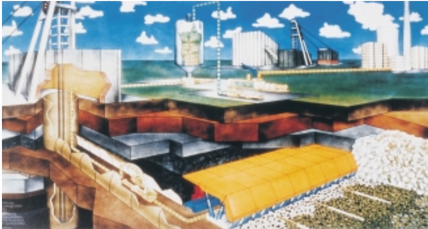
Backfilling plant using solids pumps (source: DMT in Essen, Germany)
