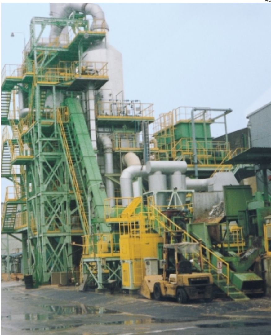
KOS solids pumps convey paper sludge into the rotary kiln. Every day more than 450 t of cardboard is produced from waste paper
