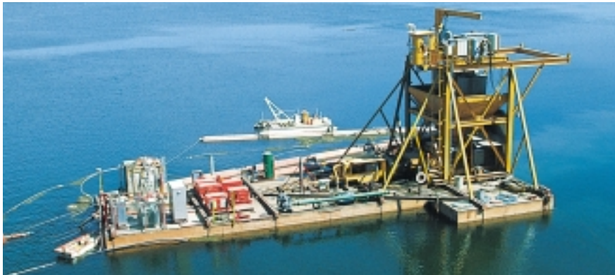
Removal of sludge from the Aswan reservoir in Egypt using the KOS piston pump
