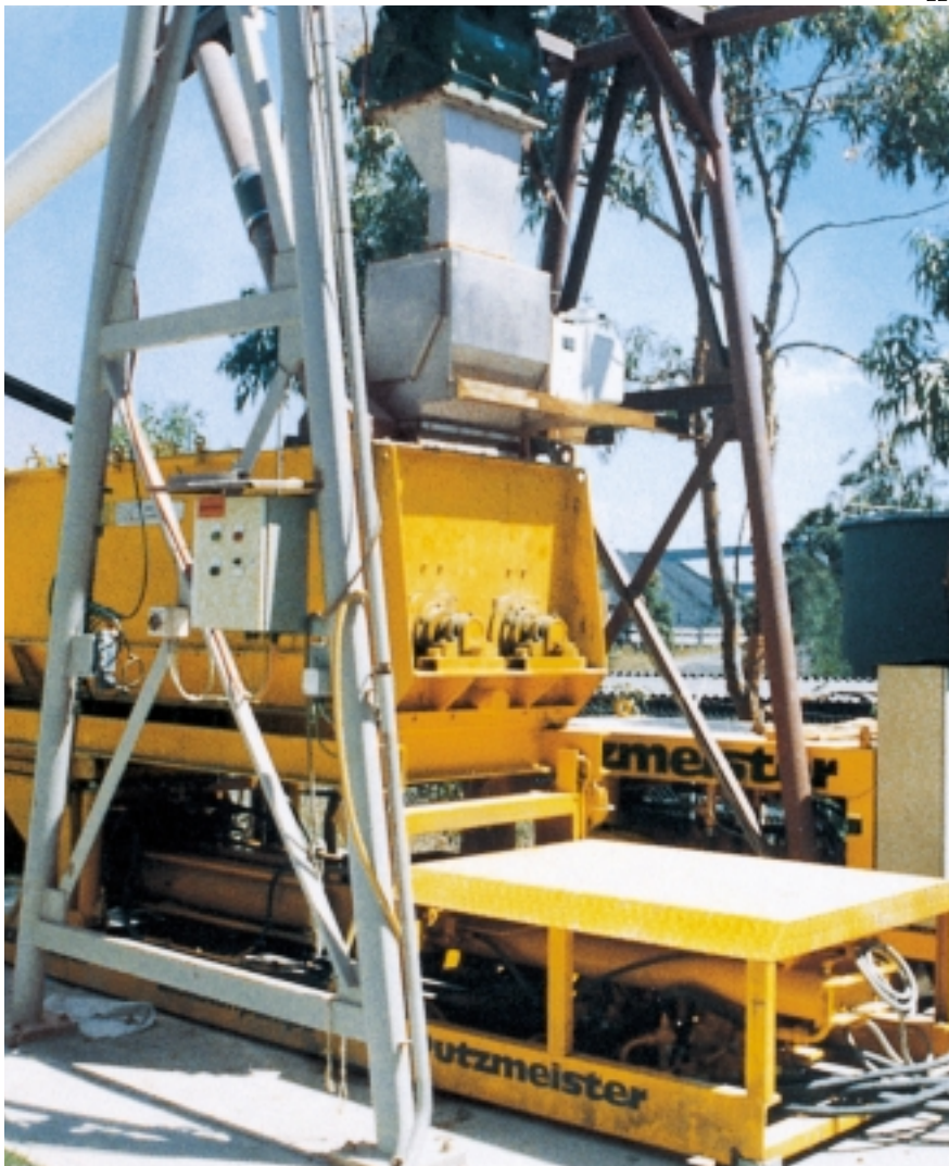
Conveying fly ash with a high solids contents of over 60% (Australia)
