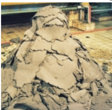
Sewage sludge dewatered by means of chamber filter presses: solids content > 35% solids
