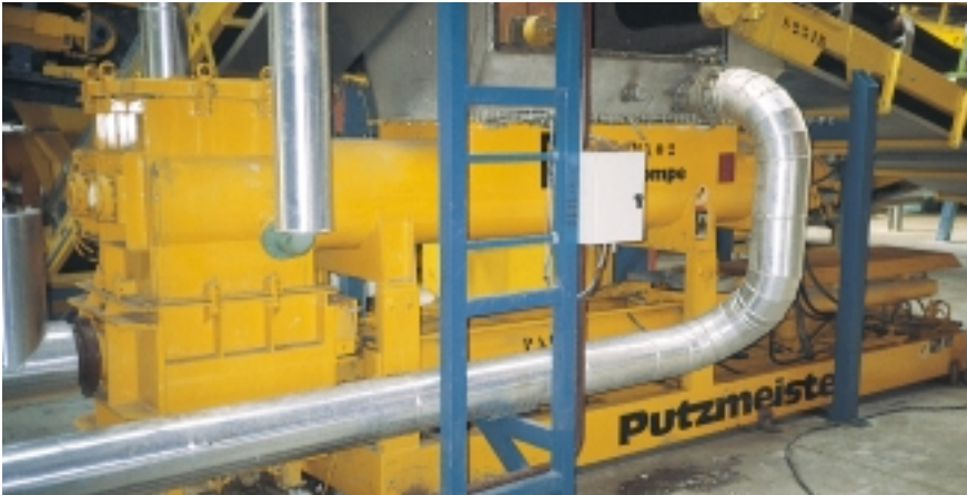
A KOS 2180 pumping organic waste at the Valorga refuse gasification plant in Amiens, France
