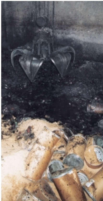
Coarse hazardous waste from the reception bunkers is fed by the grab to the EKO piston pump
