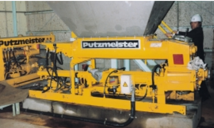
A Putzmeister KOS 1030 solids pump conveying paper sludge into the rotary kiln
