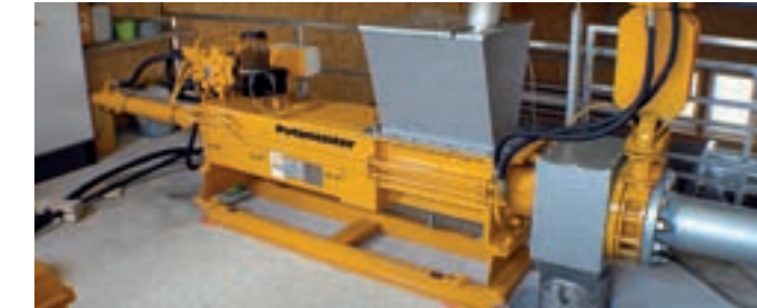
EKO 1060 PP at the biometanisation plant in Kössen (Austria) for the transportation and de-wrapping of expired food
