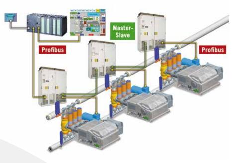
Three FELUWA Triplex MULTISAFE® pumps discharge into a common main. FELUWA pump synchronisation controls phase shifting and effectively prevents swinging up of resonances.
