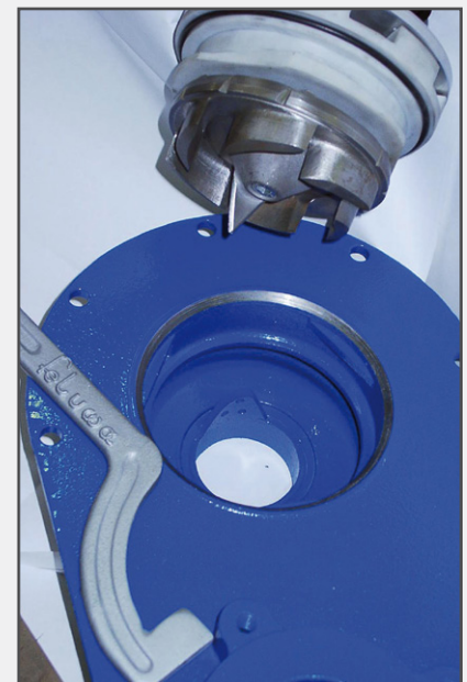
Separation of pump rotor by means of hooked spanner.
