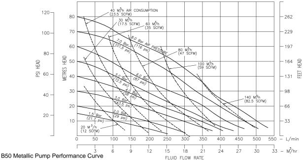
Performance based on water at ambient temperature
